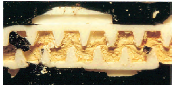
Figure 14. Dripper with calcium precipitate. The black pieces are parts of the cut-away plastic dripperline and not contaminants.
