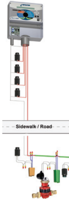
Adding 2-Wire, master valve and flow sensor using existing conventional wires
