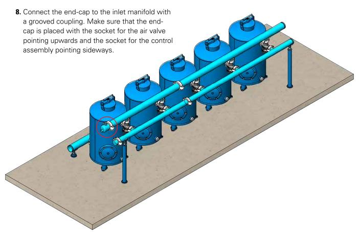
**9.** Connect the end-cap to the outlet manifold with a grooved coupling.
