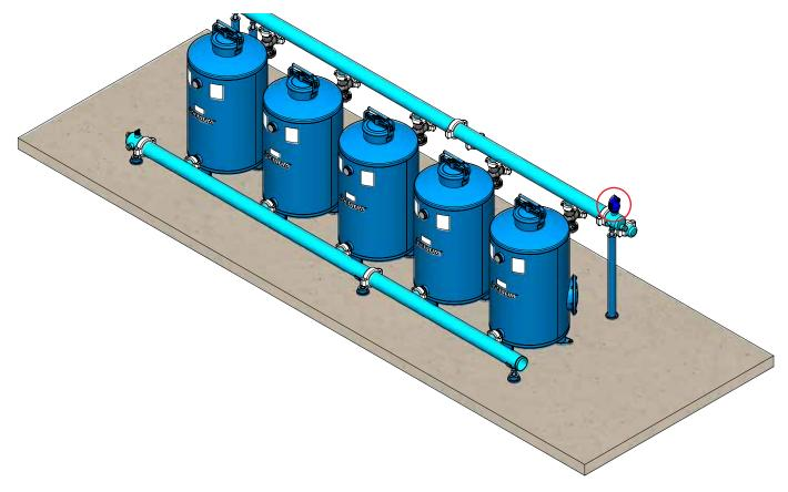
11. Connect the control assembly to the socket on the side of the inlet manifold end-cap.
