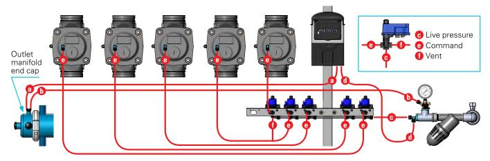
15. Connect the solenoids to the BackFlush controller expansion cards in sequence, from left to right. Red wire = + / black wire = common (inversing wire polarity will change NC to NO).
