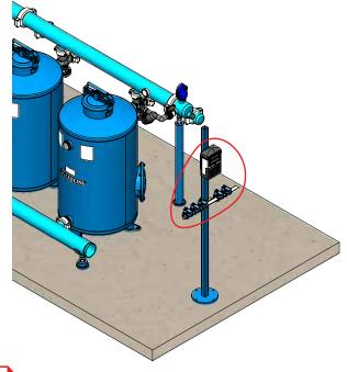
Connect the filtration system to the main line and backwash pipe with grooved couplings.
