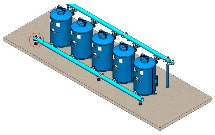
10. Connect the air valve to the socket on the top of the inlet manifold end-cap.
