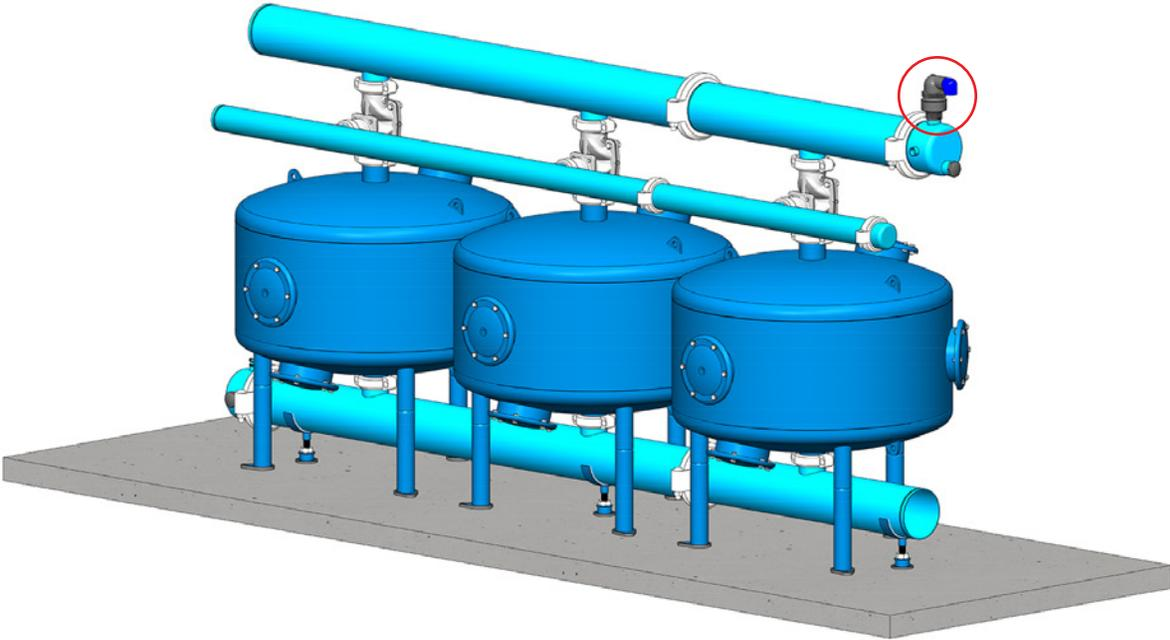
12. Connect the air valve to the socket on the top of the inlet manifold end-cap.
