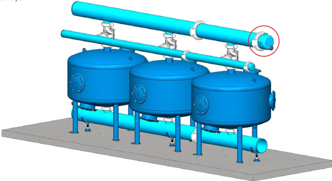
9. Connect the end-cap to the outlet manifold with a grooved coupling. Make sure that the end-cap is placed with the 1" outlet pointing upwards.
