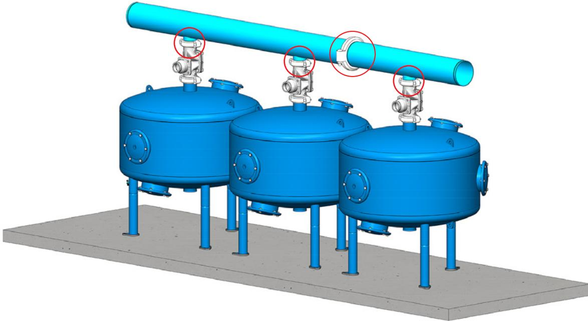
4. Connect the backwash manifold to the backwash valves and the backwash manifold sections to each other with grooved couplings.
