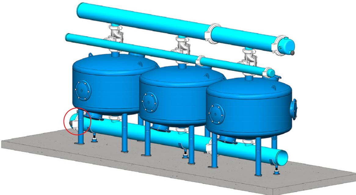
10. Make sure that all the grooved coupling connections are properly aligned.
