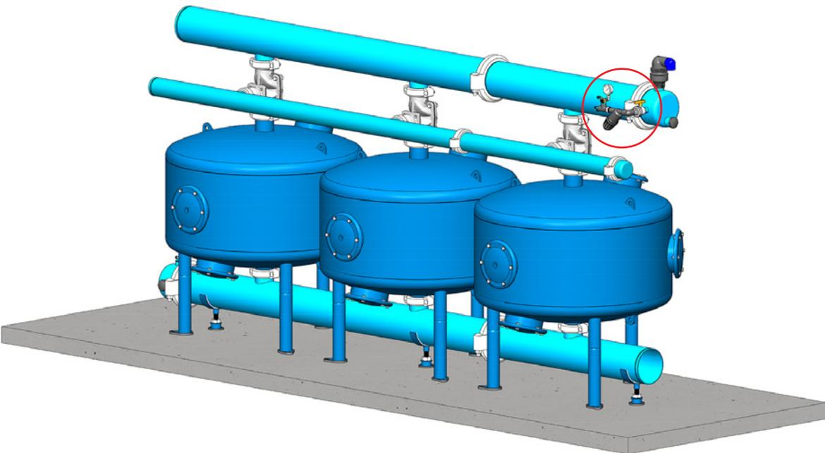
14. Place the stand of the backwash controller so that it is close to the control assembly (make sure it meets your needs for both operation and maintenance). Secure it to the concrete slab with 10 mm spreading anchor bolts.
