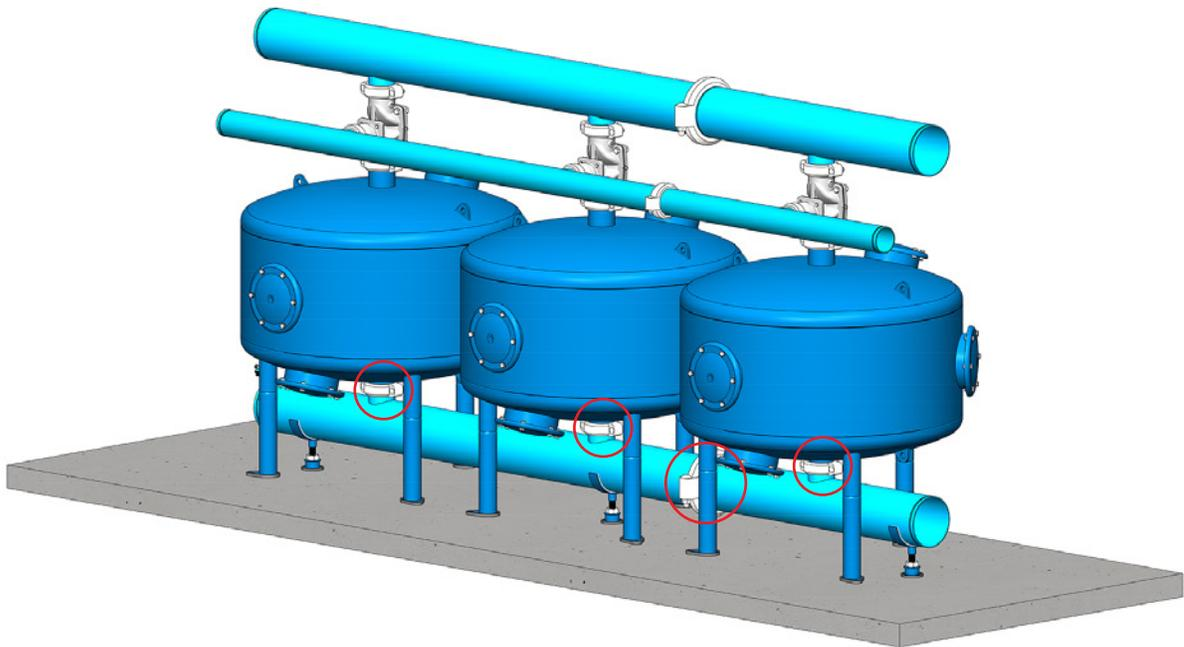
6. Check and confirm that the position of the system is where it should be relative to the inlet and outlet main pipelines. Readjust the filtration system location if needed.
