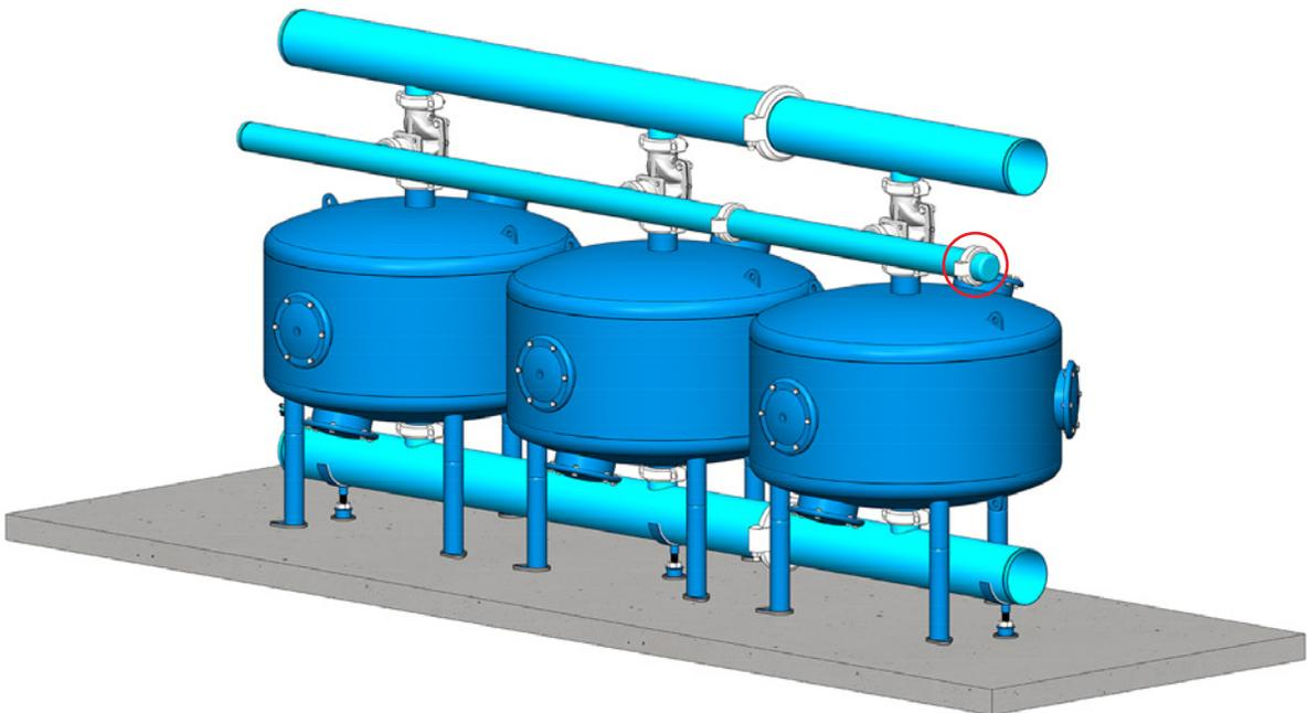
8. Connect the end-cap to the inlet manifold with a grooved coupling. Make sure that the end-cap is placed with the socket for the air valve pointing upwards and the socket for the control assembly pointing sideways.
