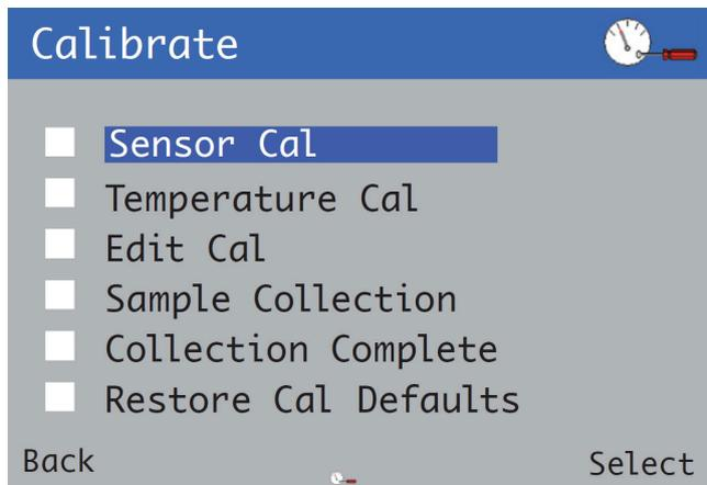
3. Use the / keys to select **Sensor Calibration** and press the key to confirm selection.
