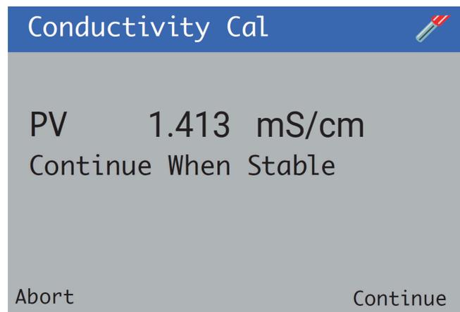
4. Confirm the displayed reading is stable and press the key.
