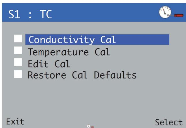
3. Use the / keys to select **Conductivity Cal** and press the key.
