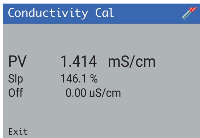
Invalid new calibration values generate an error message and the calibration value is not accepted.
