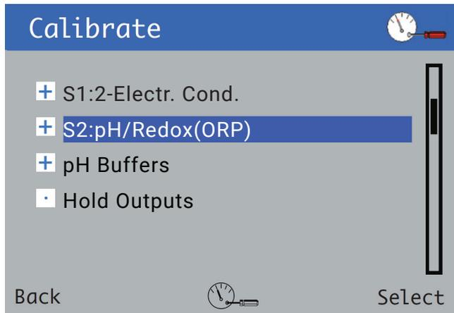
2. Use the / keys to select the sensor to be calibrated, and press the key to confirm selection.
