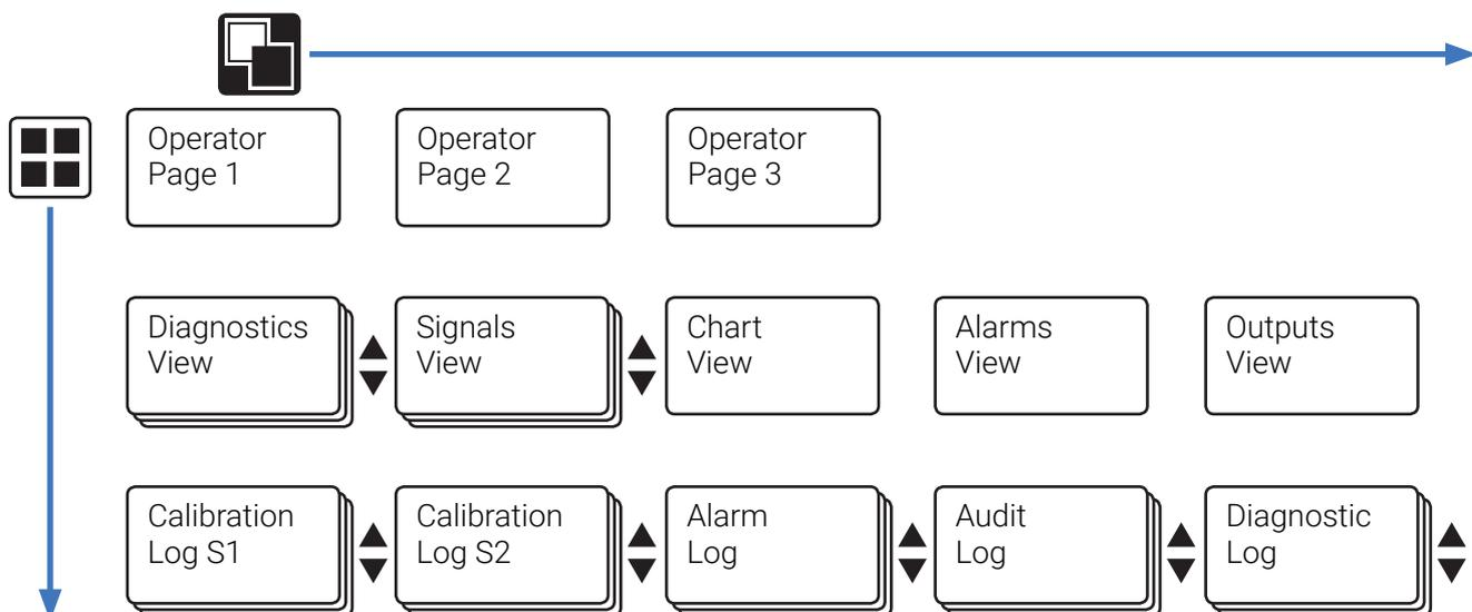
**NOTE:** The calibration log for a sensor (S1 to S2) is displayed only if that sensor is fitted.
