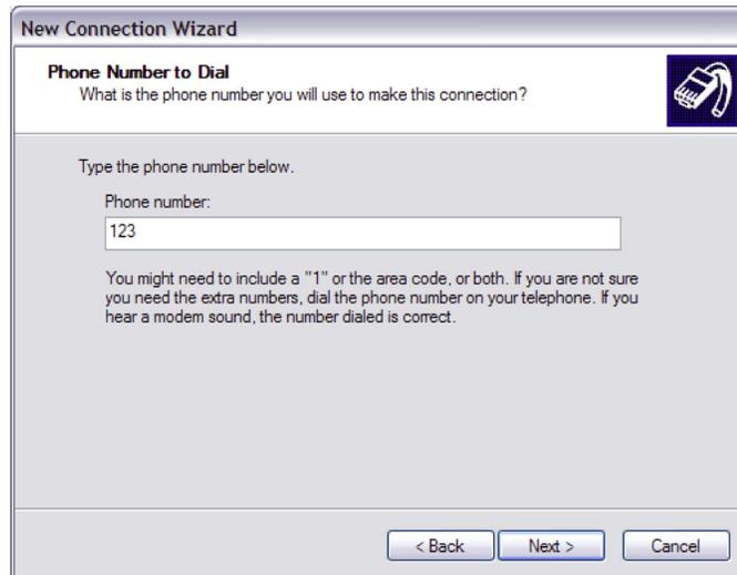
If the connection is being created for direct local access using a COM port, you should set the phone number to 123. This number will be intercepted by the unit and recognized as an attempt to connect locally.
