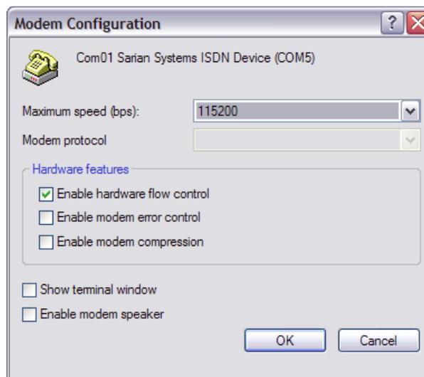
Make sure that the **Maximum speed (bps):** value is set to **115200** and that the **Enable hardware flow control** box is checked. Click **OK** when you have finished to return to the main properties dialog.
