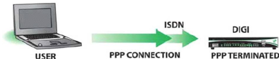
With L2TP answering the call, the router terminates the layer 2 connection only and the PPP frames are passed in an L2TP "tunnel" to another device which terminates the PPP connection. This device is sometimes referred to as a Network Access Server (NAS).
