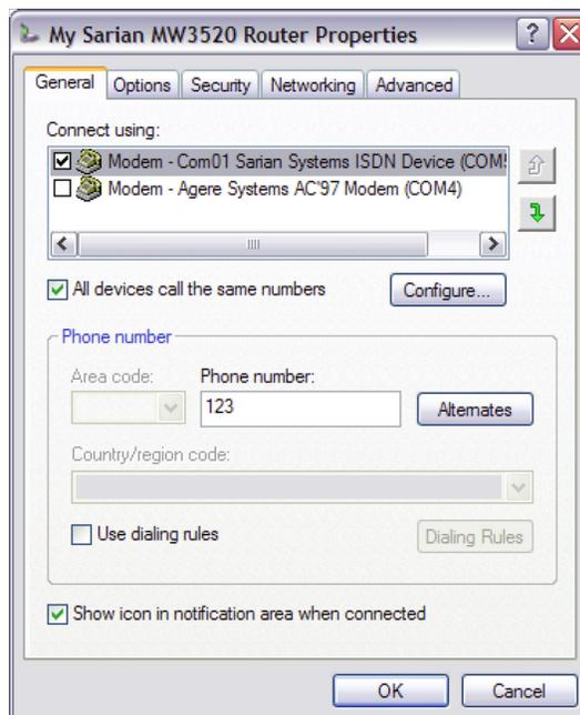
3. On the **General** tab, click the **Configure...** button to display the Modem Configuration dialog:
