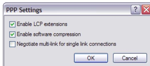
Make sure that all three options are **unchecked** before clicking **OK** to return to the **Networking** tab. In the **This connection uses the following items** list, **Internet Protocol (TCP/IP)** should be the only item that is checked. Make sure that this is the case and then click **OK** to return to the main dialog. You are now ready to initiate a connection.
