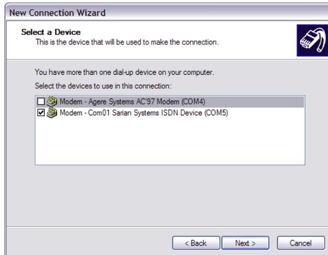
4. From the **Select a Device** dialog, select the unit you have just installed and make sure that any other devices in the list are unchecked. Click **Next >**.
