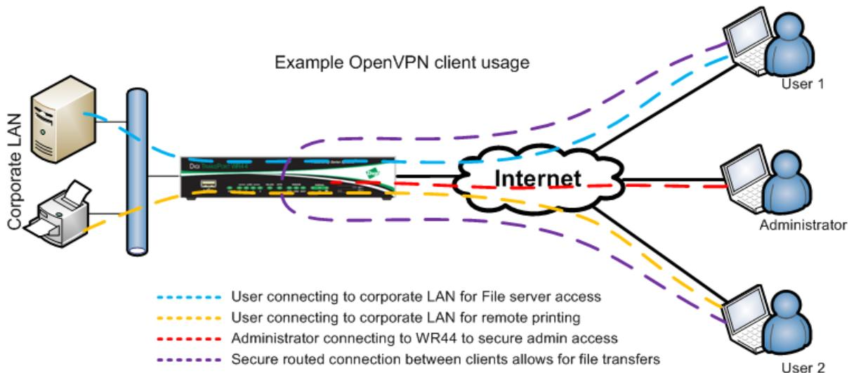
The Digi TransPort implementation of OpenVPN can be configured as an OpenVPN server (shown above) or as an OpenVPN client, connecting to an OpenVPN server.
