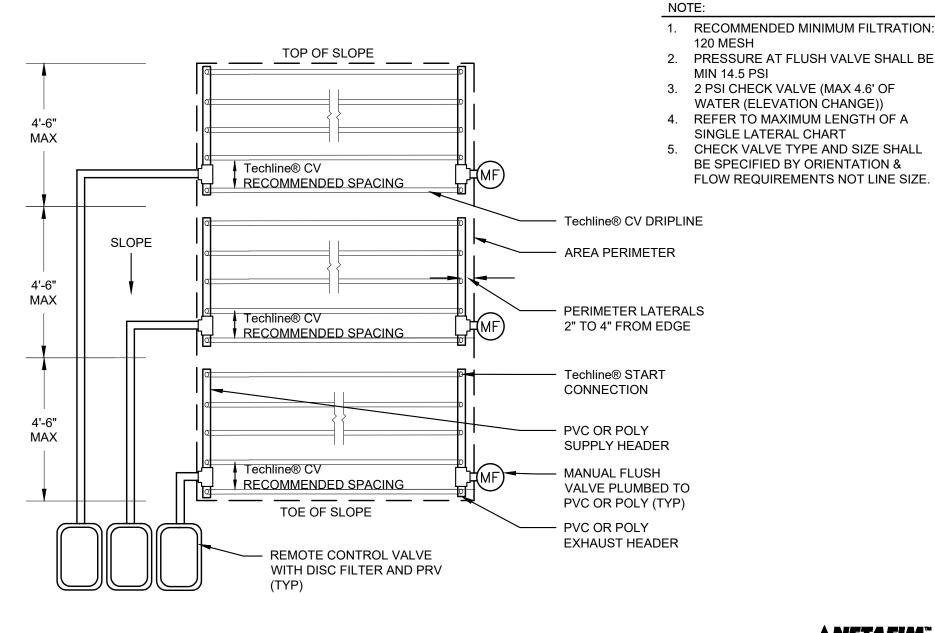
Techline® CV SLOPE LAYOUT, 3 VALVES-BOTTOM OF SLOPE
