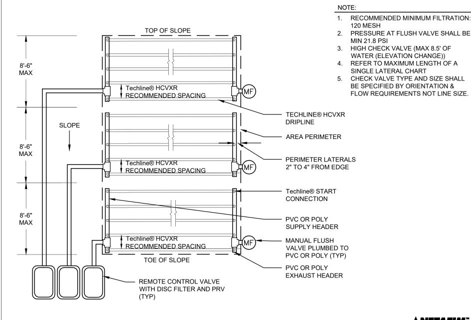
Techline® HCVXR SLOPE LAYOUT, 3 VALVES-BOTTOM OF SLOPE & NETAFIM
