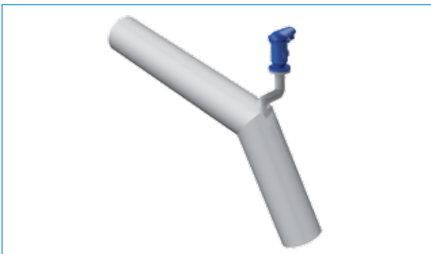
Negative breaks: increase in a downward slope
